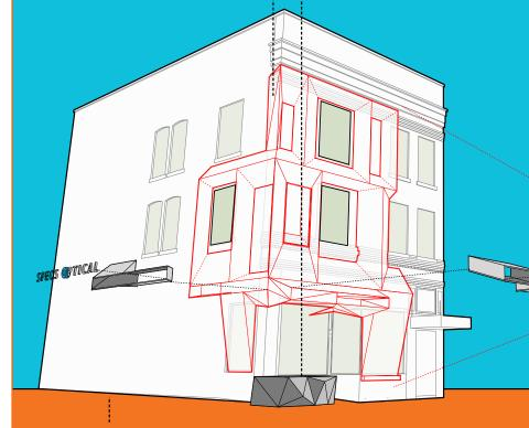
Instead of working drawings, a laser-cut scale model (1/2"=1"-0") of the skin was used as a 3-D guide to installation, with all pieces numbered in small and full scales.
